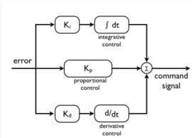
Fig. 3 PID control system
