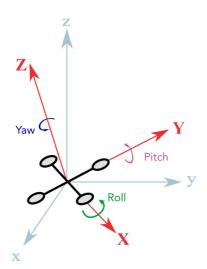
Fig. 2 Inertial Frame, Red: Body Frame
