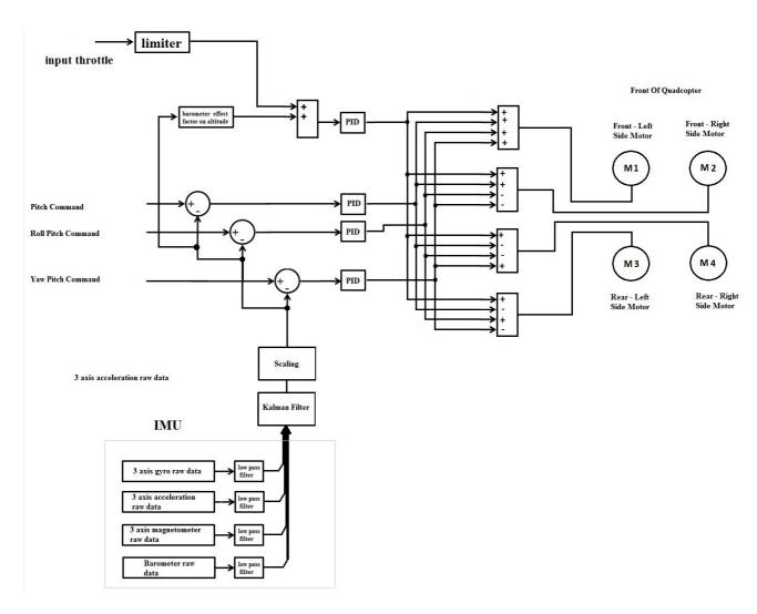
Fig. 4 Block diagram of control system
